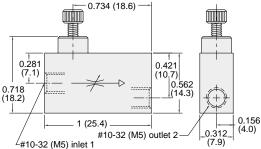
Materials: Brass body and stainless steel needle; Buna-N seals Input Pressure: 300 psig max.
